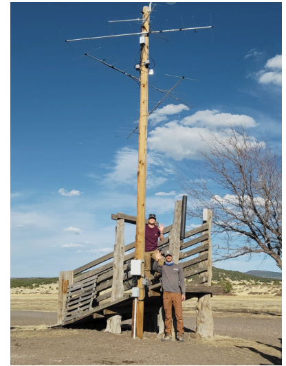
A Motus station consists of antennas mounted to a structure (in this case an old telephone pole), connected to a receiver and a computer.
