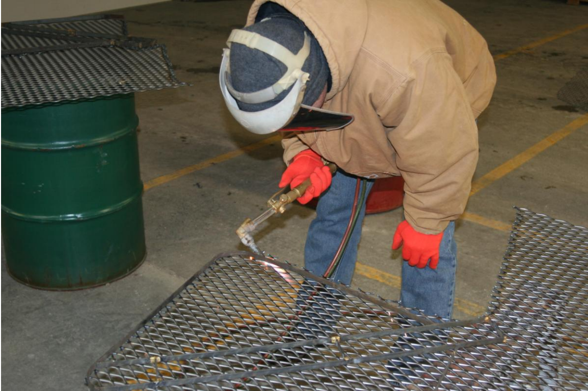
Figure 13. NPP personnel using acetylene torches to cut bulk expanded metal in the shape of wildlife escape ladders that would later be bent prior to installation in tanks.
