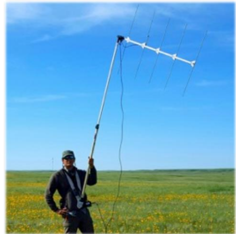
Figure 7: Bird Conservancy crew lead Sasha Robin with 5-element antenna and extension pole, used to track tagged birds. Photo by N. Guido.
